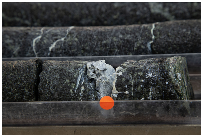
Figure 2. The MBIO sample (orange circle) is photographed before it is removed from the core. This example shows a fractured zone that was targeted for microbiological investigation. Photo credit: Erick Bravo, IODP JR50.
