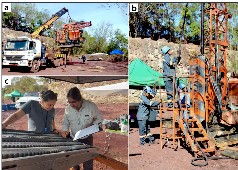
Figure 12. Photos of drilling the GRIND-ECT cores in Brazil. (a) Arrival of the drilling rig at the Sobramil site. (b) Anchoring the drilling rig at the Sobramil site. (c) Kamilla Amorim and Paulo Boggiani working on the description of the dolostone of the Bocaina Formation.
