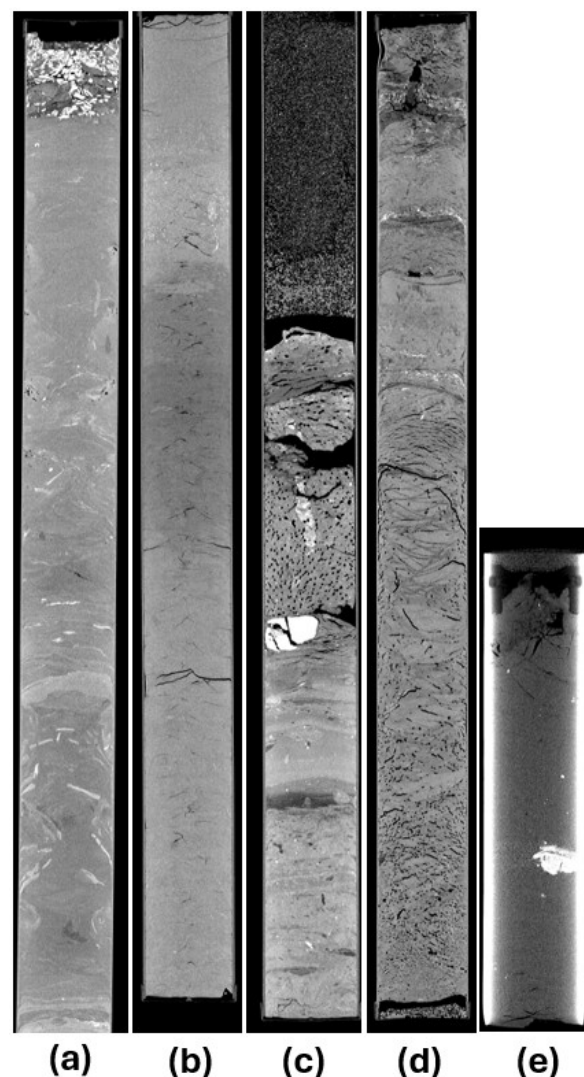
Figure 4. Selection of CT scans of core material. Visualisations are made with a greyscale ranging from 450 to 1600 HU (a–d) or 1500 to 3000 HU (e). The cores and corresponding top depths are (a) DAPGEO-02-C6 – 136.0 m b.g.l., (b) DAPGEO-02-C45 – 387.9 m b.g.l., (c) DAPGEO-02-C55 – 391.2 m b.g.l., (d) DAPGEO-02-C64 – 398.6 m b.g.l., and (e) DAPGEO-02-C70 – 402.6 m b.g.l.
