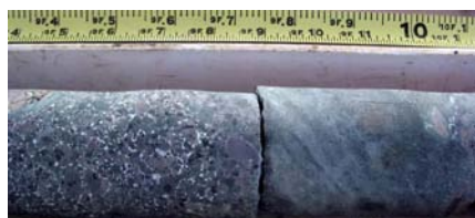
Core from 3507.6 m depth with pillow breccia clasts surrounded by a matrix of blue-green clay; beneath the breccia (left) is a layer composed almost entirely of clay.
