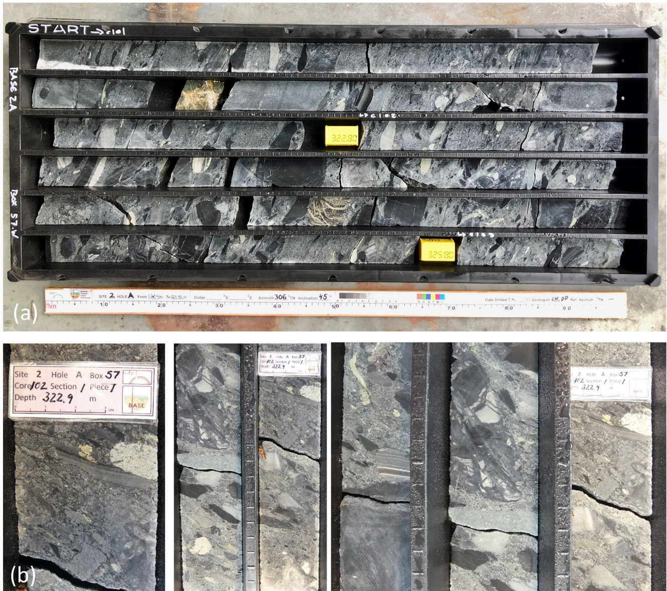
Figure 21. Examples of core photographs. (a) Slabbed and wet core of box 57 of borehole BASE 2A, showing ca. 2.5 m of core 101, all 3 m of core 102, and 0.4 m of core 103. The stratigraphic top is to the upper left. The data bar provides information about the depth, date, and staff. (b) Examples of handheld close-up photographs of the same core tray, showing textures of the cobble conglomerate and composition of individual clasts, mostly latite (“feldspar porphyries”) and chert.
