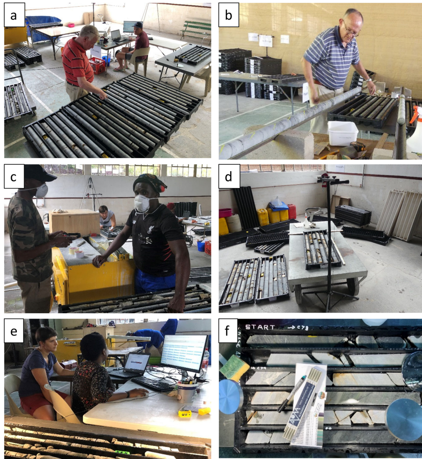
Figure 11. Stations of core processing in BIAS Hall: (a) re-packing; (b) orientation; (c) slabbing and splitting; (d) photography; (e) data entry; (f) lithological description and close-up photography.
