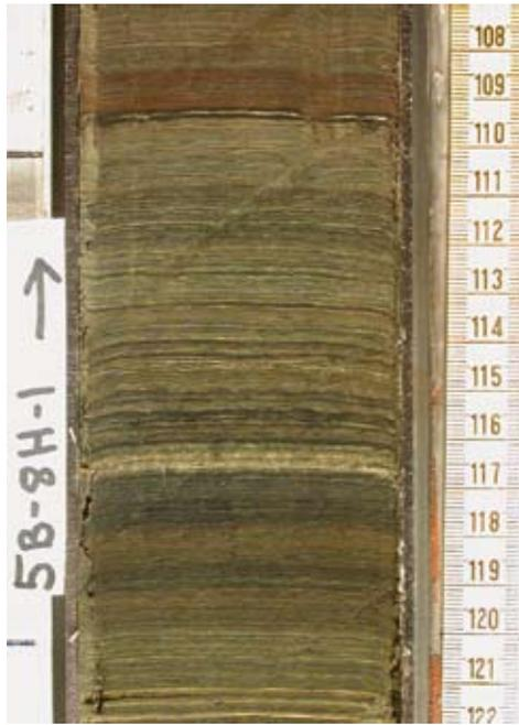
Figure 8. Laminated (and most likely varved) lake sediments from Bosumtwi core.
