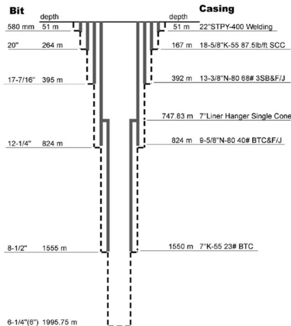
Figure 3. Casing system employed in the USDP-4 well.
