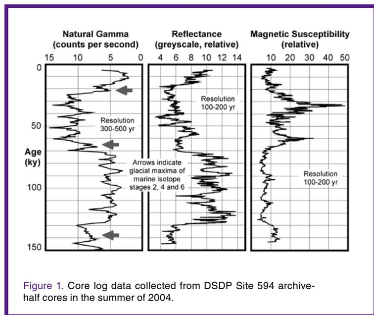
Figure 1. Core log data collected from DSDP Site 594 archive-half cores in the summer of 2004.
