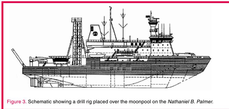
Figure 3. Schematic showing a drill rig placed over the moonpool on the *Nathaniel B. Palmer*.
