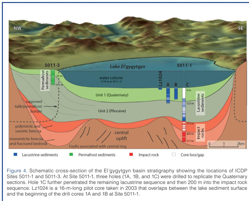
Figure 4. Schematic cross-section of the El'gygytyn basin stratigraphy showing the locations of ICDP Sites 5011-1 and 5011-3. At Site 5011-1, three holes (1A, 1B, and 1C) were drilled to replicate the Quaternary sections. Hole 1C further penetrated the remaining lacustrine sequence and then 200 m into the impact rock sequence. Lz1024 is a 16-m-long pilot core taken in 2003 that overlaps between the lake sediment surface and the beginning of the drill cores 1A and 1B at Site 5011-1.
