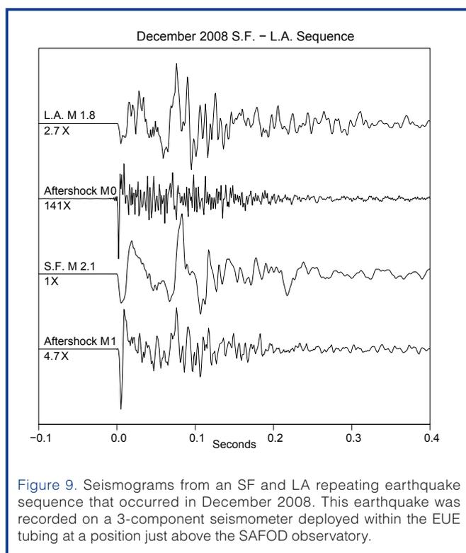
**Figure 9.** Seismograms from an SF and LA repeating earthquake sequence that occurred in December 2008. This earthquake was recorded on a 3-component seismometer deployed within the EUE tubing at a position just above the SAFOD observatory.
