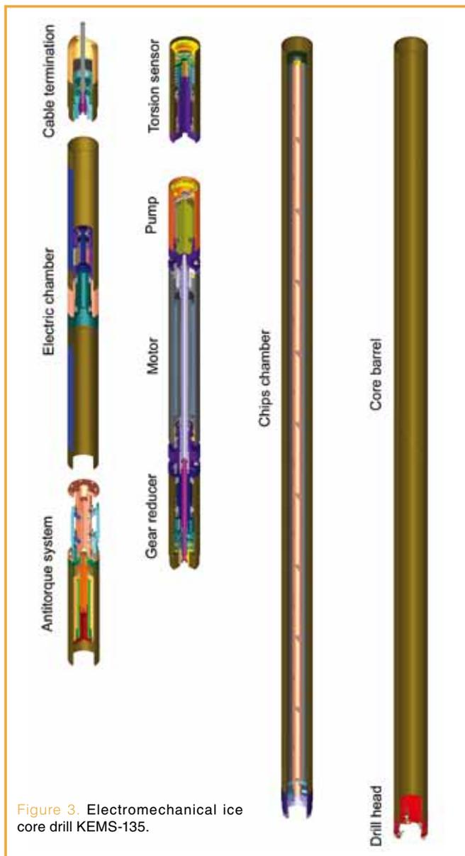
Figure 3. Electromechanical ice core drill KEMS-135.
