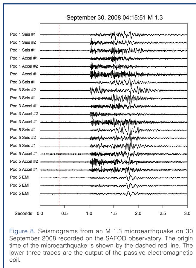
Figure 8. Seismograms from an M 1.3 microearthquake on 30 September 2008 recorded on the SAFOD observatory. The origin time of the microearthquake is shown by the dashed red line. The lower three traces are the output of the passive electromagnetic coil.
