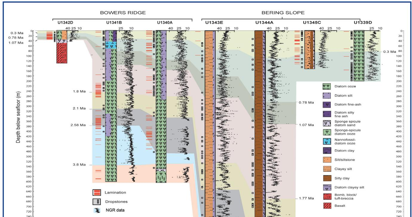
Figure 4. Lithostratigraphic summary of Exp. 323 drill sites. Natural gamma radiation (NGR: counts s<sup>-1</sup>) data are plotted in black at the right side of the lithology columns (values increase to the left). Laminations are denoted by red horizontal lines. Note that there are many different styles of laminations; future work will determine which laminations are primary features, and which are secondary.
