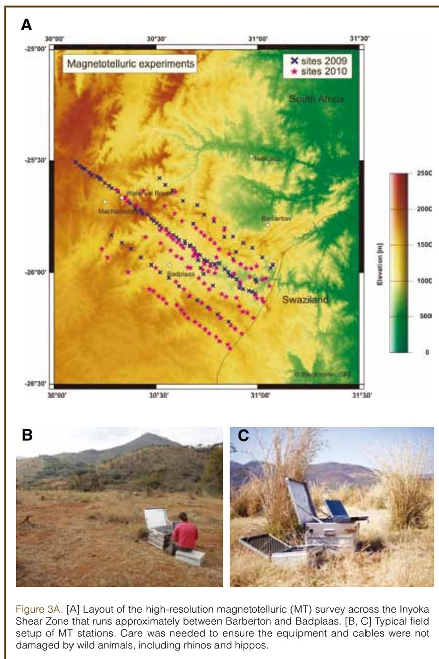
Figure 3A. [A] Layout of the high-resolution magnetotelluric (MT) survey across the Inyoka Shear Zone that runs approximately between Barberton and Badplaas. [B, C] Typical field setup of MT stations. Care was needed to ensure the equipment and cables were not damaged by wild animals, including rhinos and hippos.
