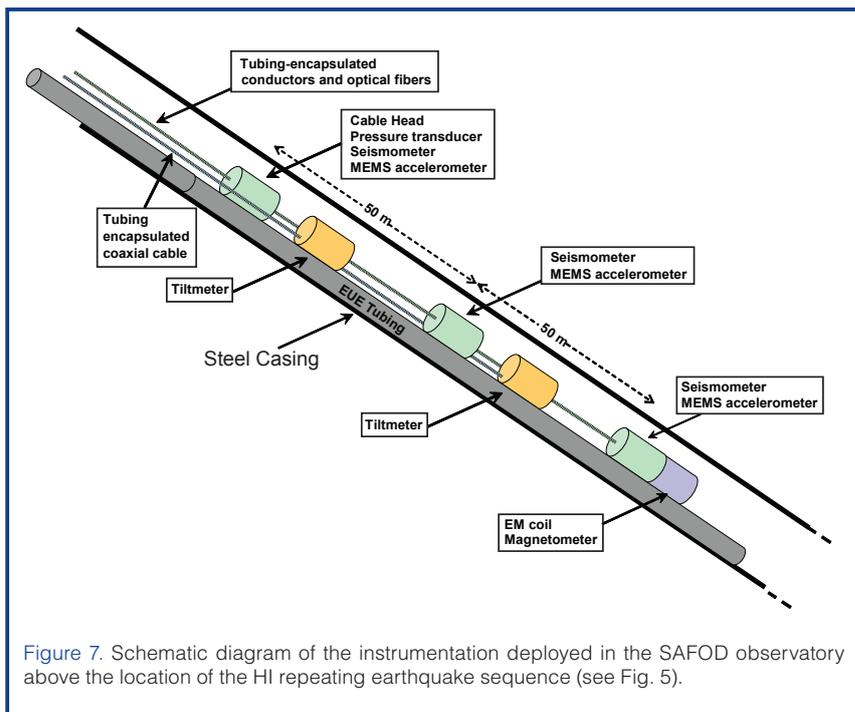
Figure 7. Schematic diagram of the instrumentation deployed in the SAFOD observatory above the location of the HI repeating earthquake sequence (see Fig. 5).
