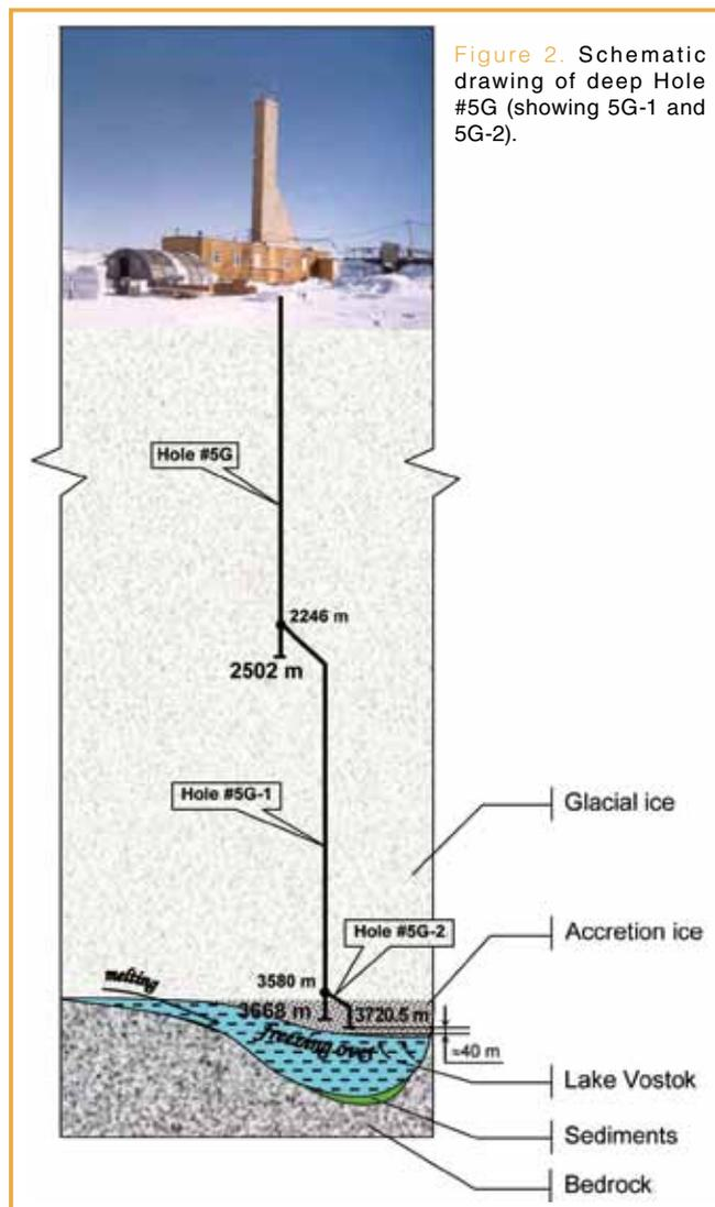
Figure 2. Schematic drawing of deep Hole #5G (showing 5G-1 and 5G-2).
