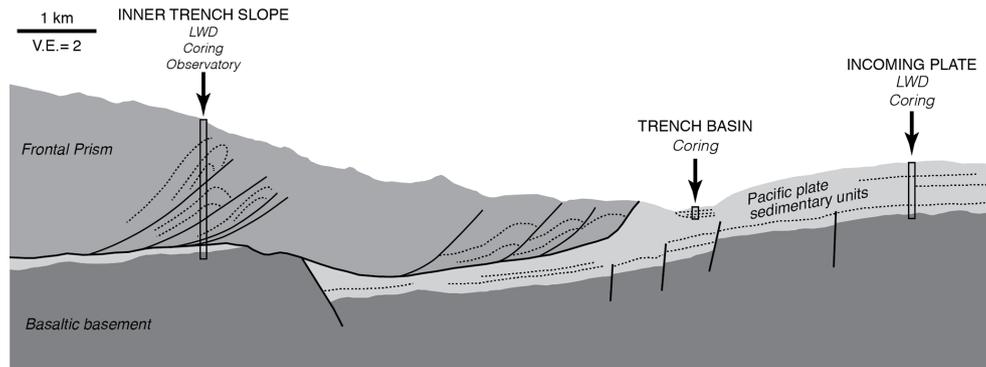
**Figure 2.** Schematic section through the frontal prism, trench and incoming section showing the framework for the two proposed trench normal transects, locations of the holes and list of target data for each hole (dashed lines represent possible bedding attitudes; solid lines are possible faults; structure based on Nakamura et al., 2013).
