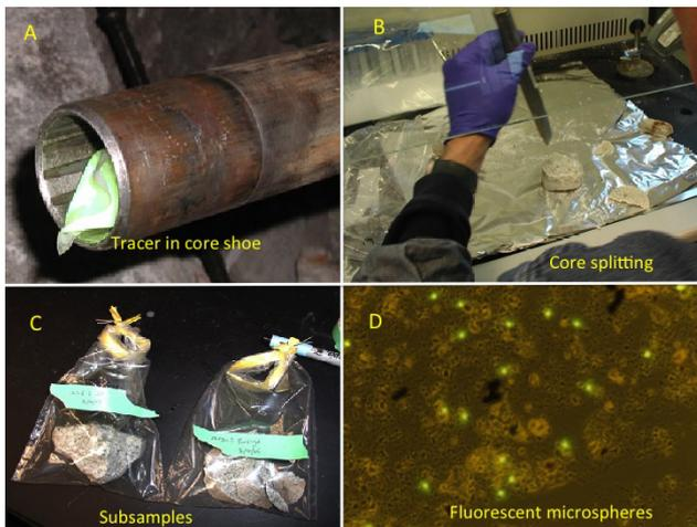
**Figure 3.** Use of tracers and subcore sampling for geomicrobiological sampling in a granitic subsurface environment (Sahl et al., 2008). (a) Fluorescent microbead tracers deployed in the core shoe, (b) subcore sampling using a hammer and chisel in a laminar flow hood, (c) subcore samples in Whirl-Pak® bags, and (d) fluorescent microbead tracers in drilling mud, viewed by epifluorescence microscopy.
