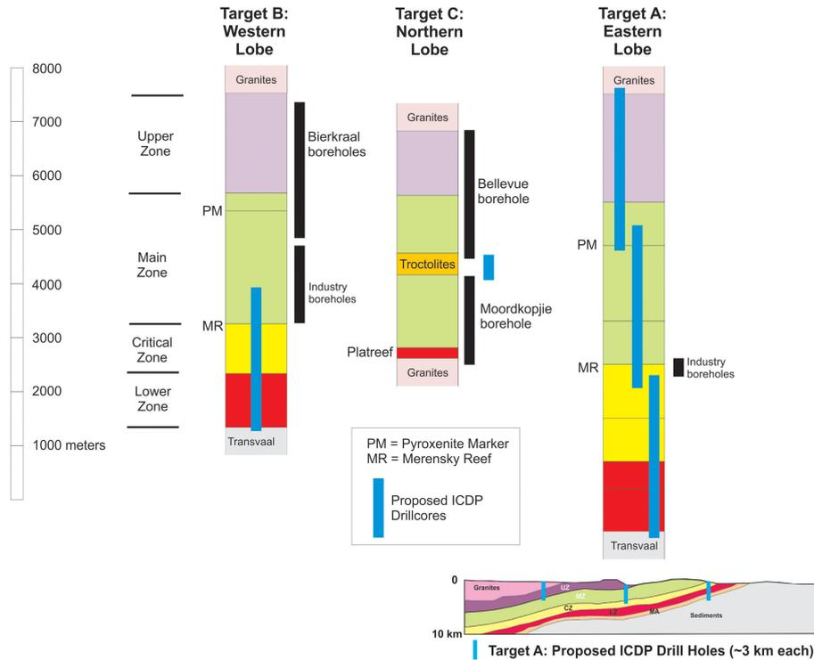
**Figure 3.** Schematic stratigraphic sections of the Bushveld lobes illustrate ICDP targets A, B and C. The cross section of the eastern lobe (right) explains the staggered-hole concept for target A (see text).
