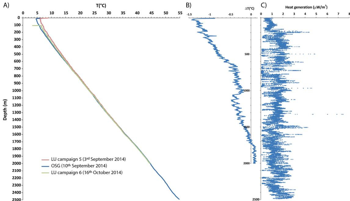
**Figure 11.** (a) Post-drilling temperature logs. Note gradual cooling (i.e. thermal re-equilibration) of the uppermost section of the borehole early in September 2014. The log measured in October is affected by post-drilling operations. (b) Temperature variations ( $\Delta T$ ) in the COSC-1 drill hole from 3 until 10 September 2014. (c) Heat generation rates as derived from the spectral gamma log measured in the COSC-1 drill hole.
