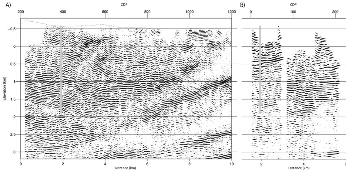
**Figure 10.** Seismic data from the pre-drilling seismic survey (a) as in Hedin et al. (2012) (b) reprocessed with a 3-D geometry over the crooked acquisition line. The grey vertical line indicates the location of the COSC-1 drill hole.
