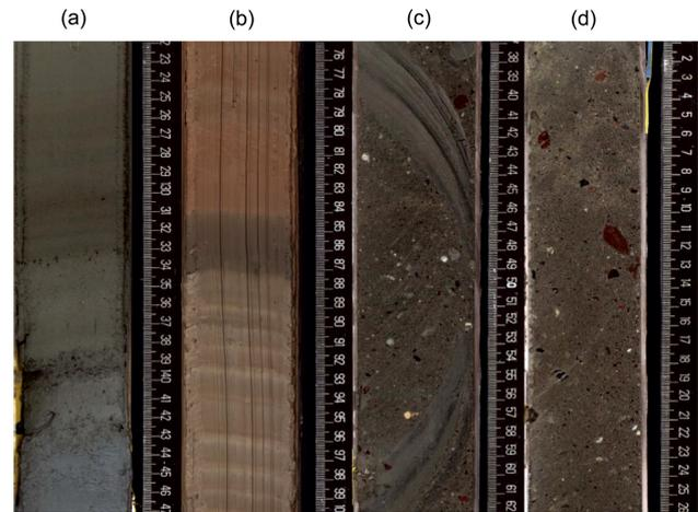
**Figure 6.** Han  Bay, site M0064. Examples of varved glacial clay (a and b) and diamicton (c, d). The greyish brown unit between 84 and 87 cm separating the two different types of varved glacial clays in section b have an age of  $45\,700 \pm 1500$  cal yr BP.
