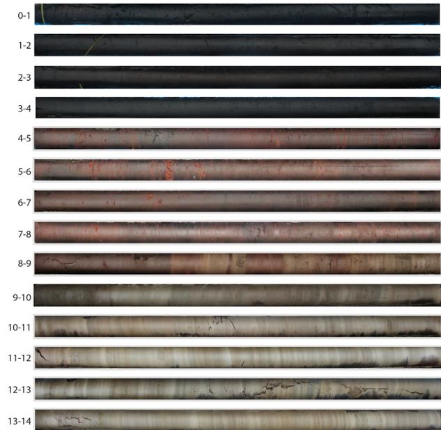
**Figure 4.** Sediments of the 14 sections of core CO 14-1 showing grey lacustrine deposits below 9 m depth, a transition between peat and lacustrine deposits between 9 and 8 m, and peat in the upper section.
