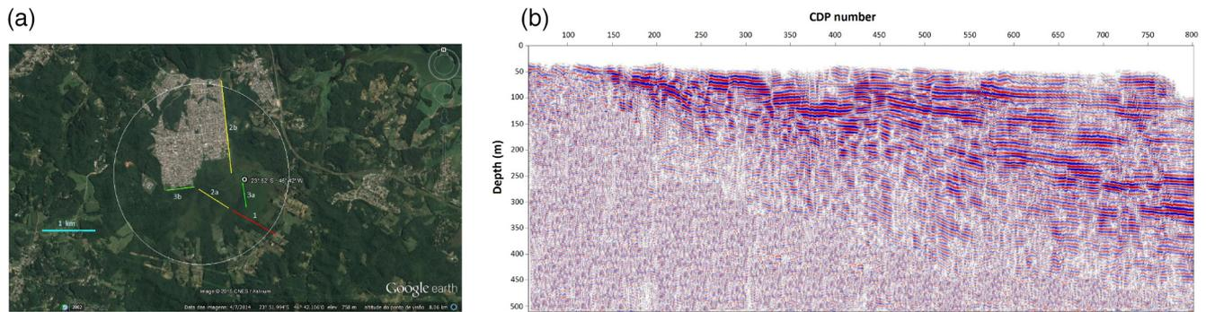
**Figure 5.** (a) Satellite view of the structure of Colônia showing the location of the 2010 seismic section (red line) and the sections planned for 2015. (b) Results of the 2010 seismic section along the Colônia structure (common depth point (CDP) trace interval = 1 m). The bright red and blue colours show the uninterpreted sedimentary infill of the basin (from Riccomini et al., 2011).
