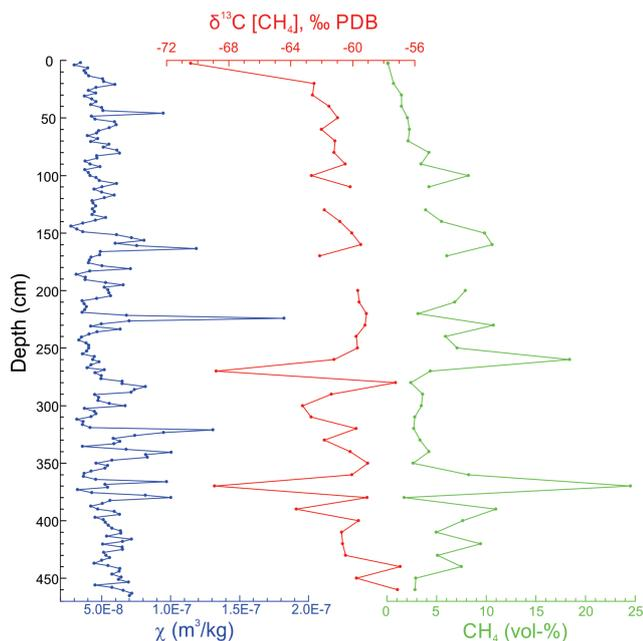
**Figure 6.** Low-field magnetic susceptibility by mass normalized of sediments and concentration  $\text{CH}_4$  (vol-%) and stable carbon isotopes  $\delta^{13}\text{C}$  [ $\text{CH}_4$ ] ‰ PDB in pore waters of XC05 sediment core. Data plotted as a function of depth.
