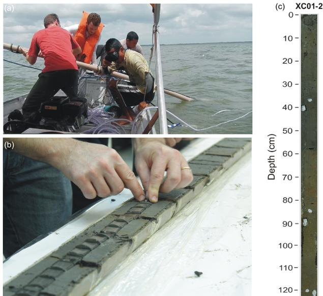
**Figure 5.** (a) Retrieving of the XC03 core during November of 2014. (b) Sampling of the XC05 core (470 cm) for magnetic analysis. This core is composed of homogenous organic muddy sediments. (c) Sediment column of the XC01-2 core, with a bottom sand layer covered by dark gray to brown muds.
