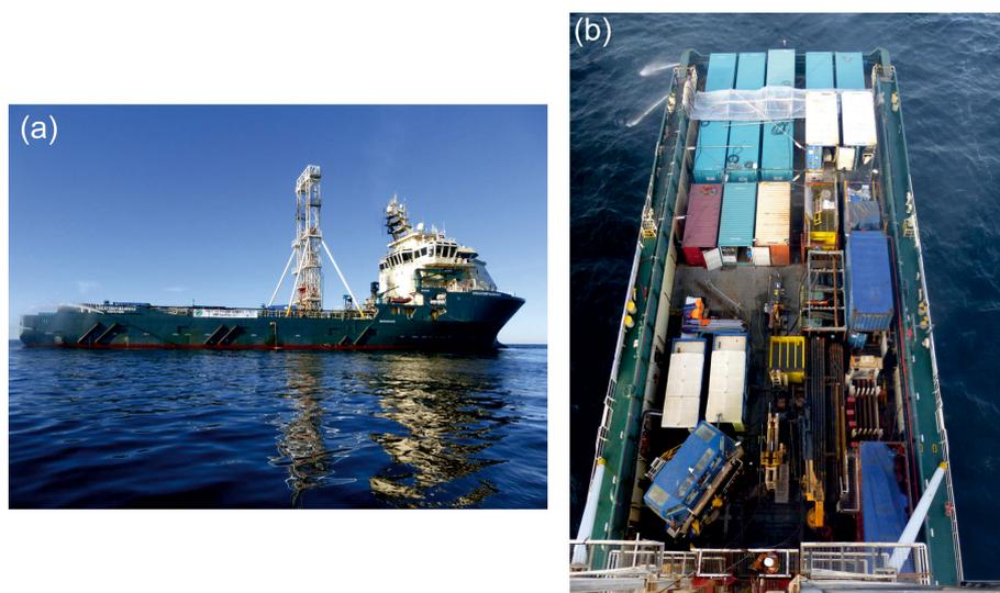
**Figure 3.** (a) The geotechnical vessel, *Greatship Manisha* (of Singapore) equipped with a drilling derrick. (b) View from the derrick over the drill deck at mid-ship and the “science garden” to the aft. Image copyright ECORD/IODP.
