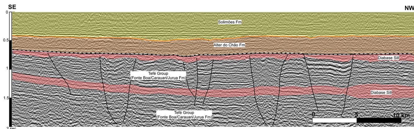
**Figure 3.** Seismic reflection profile from the Solimões Basin (location of line shown in Fig. 1). Here, the Alter do Chão Formation is illustrated to be Cenozoic (Caputo, 2011), not Cretaceous, as previously believed. Multiple diabase sills and interbedded sediments unconformably underlie Cenozoic sediments in this region. The proposed (SB) drill hole will encounter the same stratigraphic column as shown in the seismic line, but is located more accessibly on the Rio Juruá.
