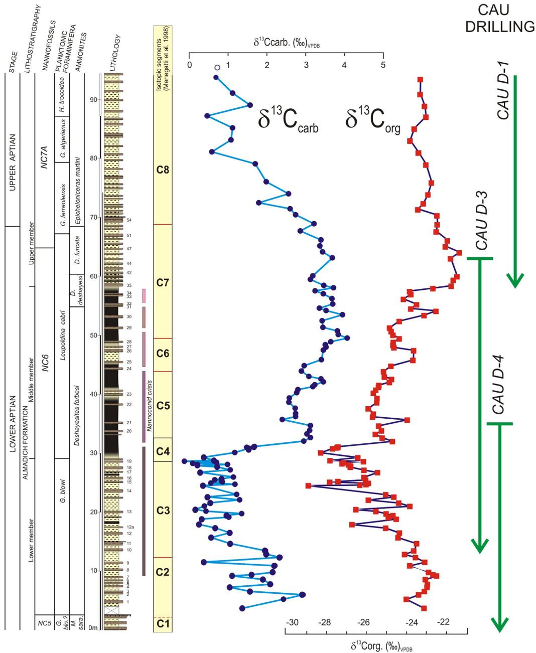
**Figure 3.** Stratigraphy of the Cau section: lithostratigraphy, biozones, and bioevents together with bulk carbonate (dark blue circles) and total organic matter stable carbon isotopes (red squares) (modified from Naafs et al., 2016). Isotope segments according to Menegatti et al. (1998). The parts of the succession recovered by each of the three drillings are shown to the right.
