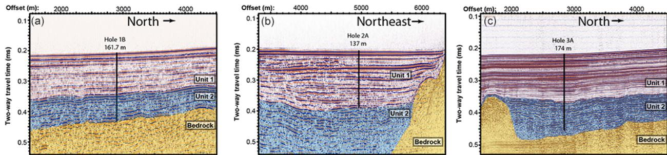
**Figure 4.** Expanded seismic reflection sections over the TDP core Sites 1 (a), 2 (b), and 3 (c), with seismic Units 1 and 2, and bedrock labeled. Black lines show the positions and depths of TDP-TOW15-1B, TDP-TOW15-2A, and TDP-TOW15-3A.
