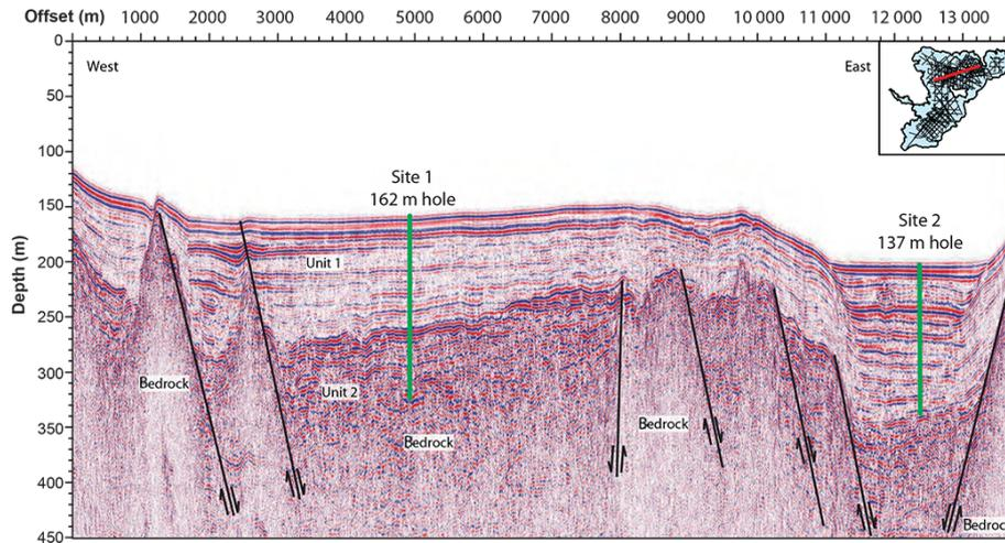
**Figure 3.** Seismic reflection profile oriented WSW–ENE over Lake Towuti’s northern basin (see inset for line position) crossing TDP Sites 1 and 2. Thick green lines show the borehole depths for TDP-TOW15-1B and TDP-TOW15-2A. Seismic Units 1, 2, and bedrock are labeled, and major faults are indicated by thin black lines.
