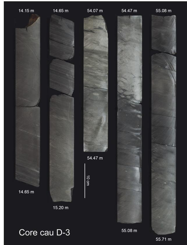
**Figure 5.** Massive and laminated, lightly bioturbated, facies of D-3 core between 14.15 and 15.20 m depth, and bioturbated facies of D-3 core between 54.07 and 55.71 m.
