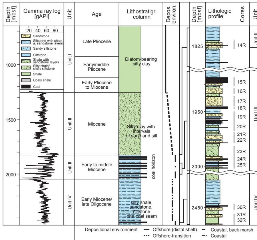
**Figure 2.** Lithologic profile of Hole C0020A based on macroscopic observation of cuttings (middle and right column) and cores (right column) recovered during Expedition 337. Gamma-ray log and positions of spot-cores are also plotted. This figure is slightly modified from Fig. 2 in Gross et al. (2015), and reprinted with permission from Elsevier.
