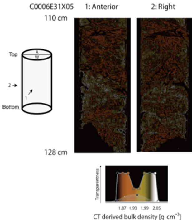
**Figure 6.** Bulk density distributions converted from the CT value for section C0006E31X05 110–128 cm. Two cross sections through the centre of the core are presented. A 3-D distribution of this section is presented as a movie in the Supplement.
