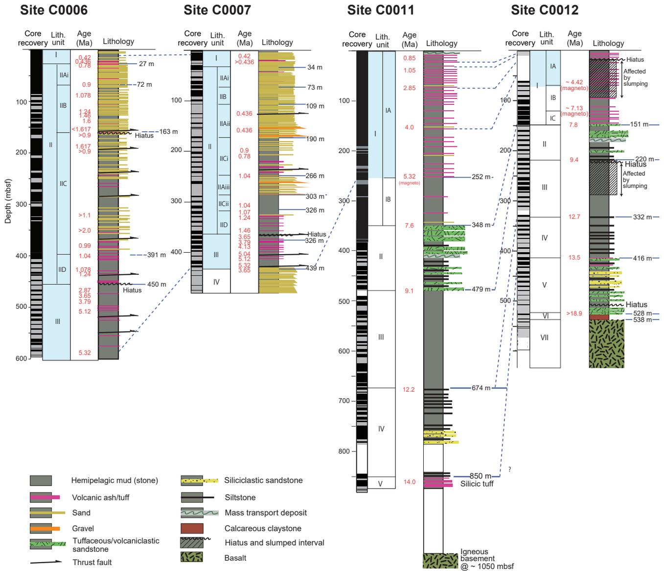
**Figure 3.** Lithological section across the Nankai frontal prism (Sites C0006 and C0007) and the input sites (C0011 and C0012). The columns at each site show core recovery, lithologic units, sedimentary age, and lithology distribution modified from Kinoshita et al. (2009), Strasser et al. (2014), and references therein.
