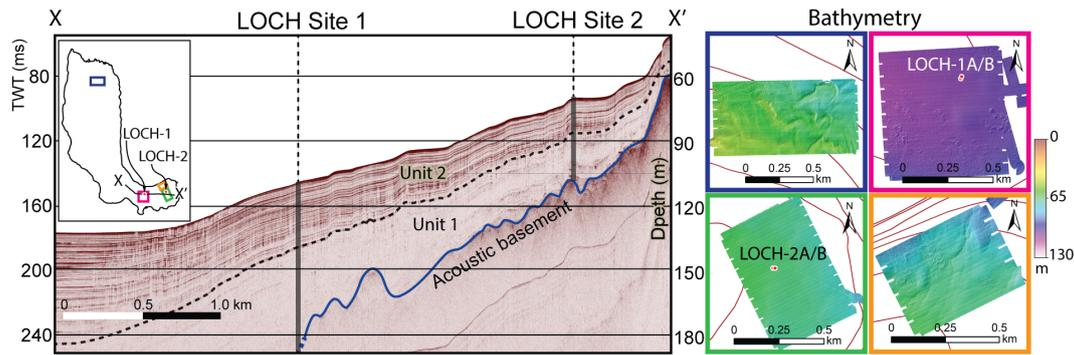
**Figure 3.** Seismic (boomer) reflection profile and sonar data from Lake Ohau showing the progressive thickening of the post-glacial sequence toward the central lake basin. The inset map shows the location of profile X–X′, LOCH drill sites (red dots), and bathymetric surveys (coloured squares correspond to data shown at the right of the figure).
