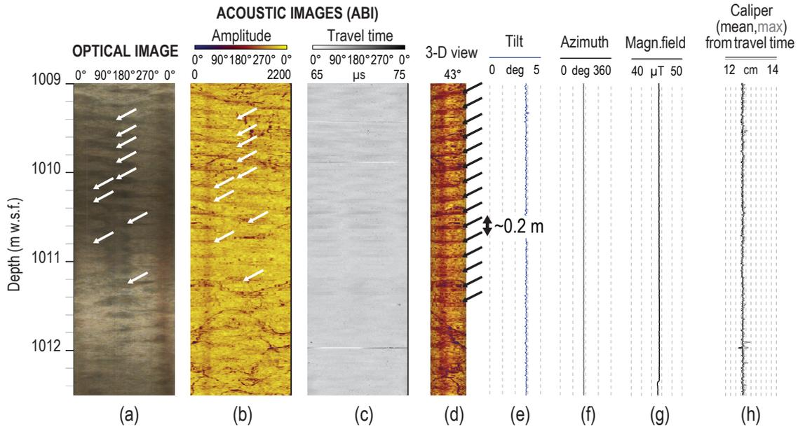
**Figure 7.** Drilling-induced helical marking on the borehole wall, evidenced by helical stripes (arrows) on both the optical and acoustic borehole images. m w.s.f. is meter wireline depth below seafloor.
