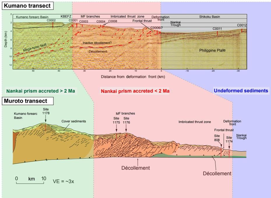
**Figure 2.** Synthesis structural cross sections across the Nankai accretionary prism along the Kumano and Muroto transects. See location in Fig. 1. The colors are the same as Fig. 1 and refer to the stage of evolution of the deformation within the Nankai Trough, namely, blue: non-accreted sediments; red: accreted sediments less than 2 My ago; green: accreted sediments more than 2 My ago. Modified from Moore et al. (2001) and (2009).
