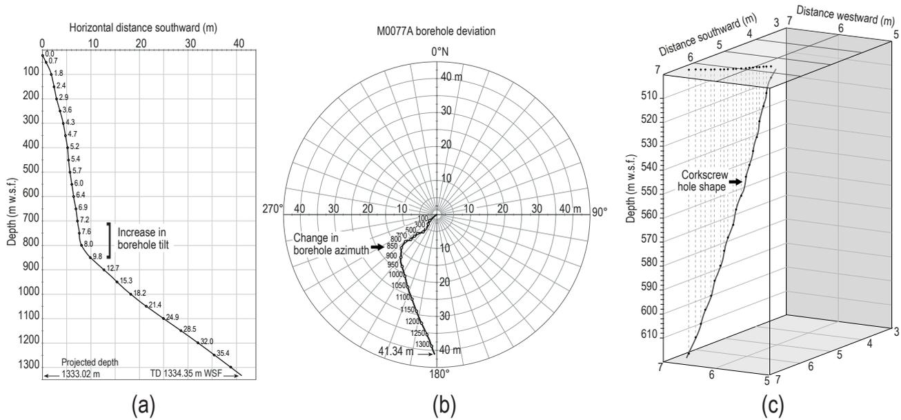
**Figure 2.** (a) true vertical depth and southward deviation of Hole M0077A. Note the increase in borehole tilt between 750 and 850 m w.s.f. (b) top view projection of the borehole path (modified from Gulick et al., 2017). Note the change in hole direction from southwest to southeast between 800 and 950 m w.s.f. (c) zoom on the 500–610 m w.s.f. interval in post-impact carbonates illustrating a corkscrew borehole shape. m w.s.f. is meter wireline depth below seafloor.
