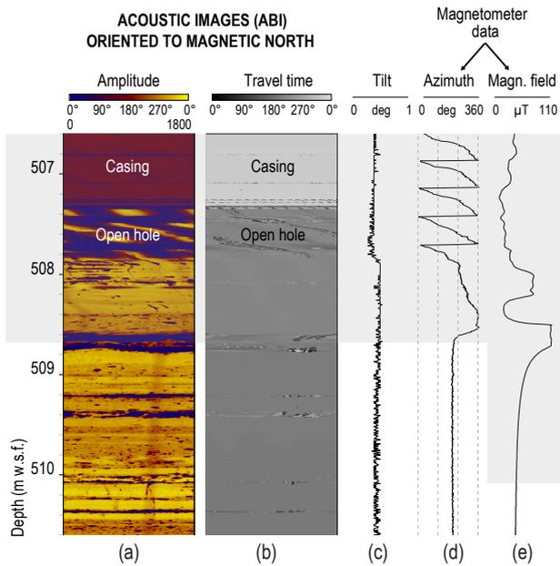
**Figure 3.** Commonly encountered magnetometer perturbation observed when approaching the entrance of a steel pipe or casing as the presence of metal close to the tool perturbs the magnetic field (d, e). As a result, the acoustic borehole image is incorrectly displayed and oriented (a, b). Grey shaded area indicates the zone under casing influence, overestimated here (see discussion in Sect. 3.1). m w.s.f. is meter wireline depth below seafloor.
