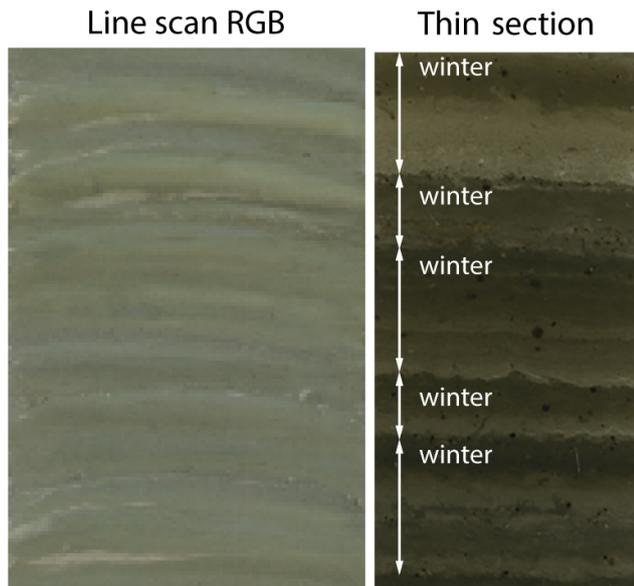
**Figure 2.** Line scan image from a 6 m long Mackereth core recovered from the sedimentary section near site MS-3. A petrographic thin section from the same core highlights sedimentary couplets that include lighter (summer) and dark (winter) layers.
