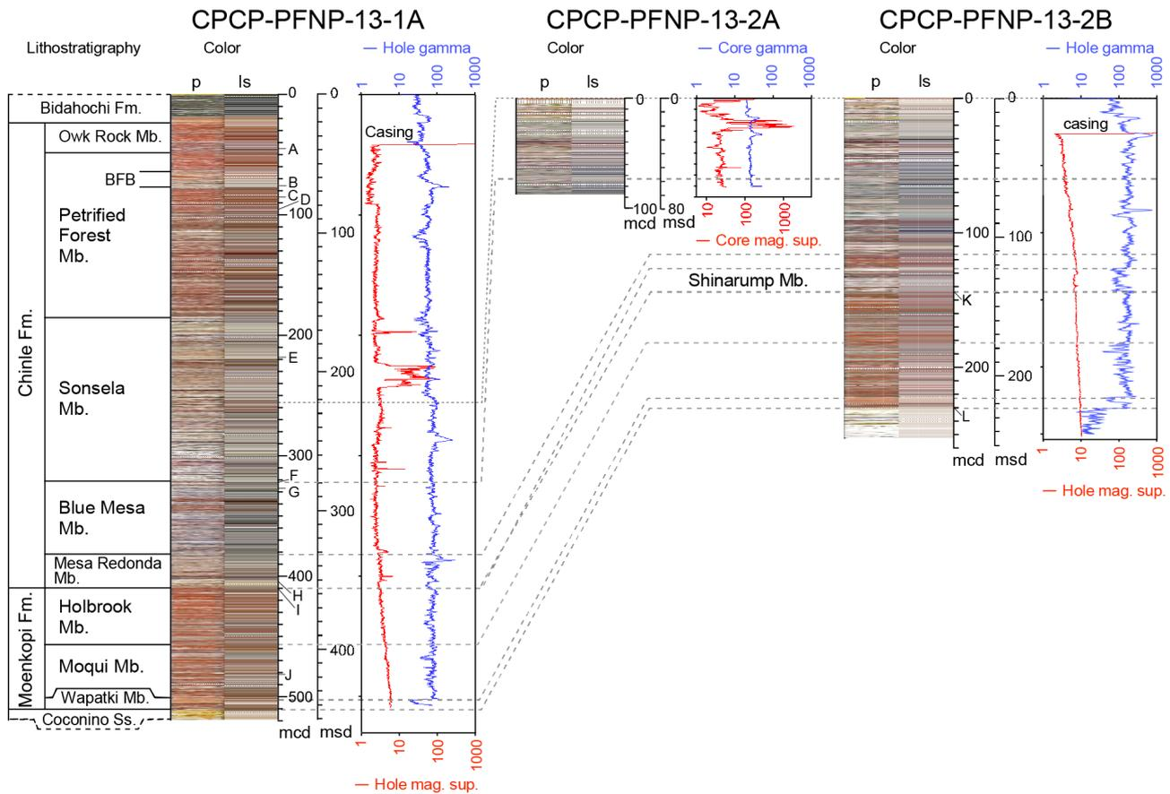
**Figure 6.** Lithologic logs, compressed photographs (p), line-scan images (ls), natural gamma, and magnetic susceptibility, for each of the cores and holes drilled during the CPCP. Letters A–K refer to core segment photographs in Fig. 8. Abbreviations for the core depths are mcd, meters core (or hole) depth; msd, meters stratigraphic depth of a core or hole with  $msd = 0.866 \cdot mcd$  in 1A,  $msd = 0.858 \cdot mcd$  in 2A, and  $msd = 0.969 \cdot mcd$  in 2B.
