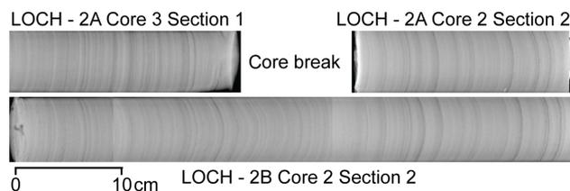
**Figure 5.** X-ray images showing 10 cm core loss at run break in LOCH-2A and recovery of the missing section in offset hole LOCH-2B (up to right). Distinct layers can be correlated between cores at mm scale from each site using visual and statistical techniques.
