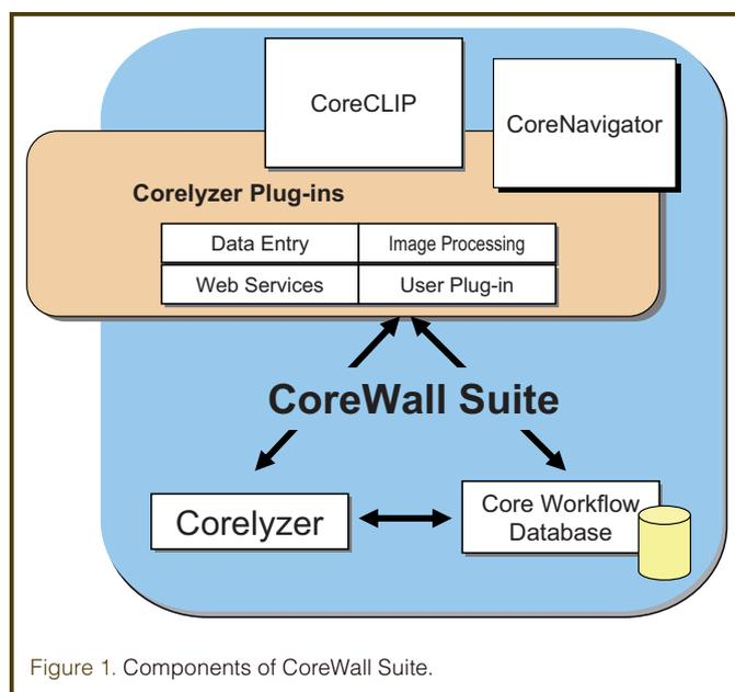
Figure 1. Components of CoreWall Suite.
