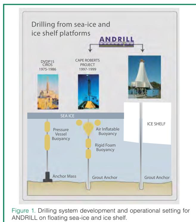
Figure 1. Drilling system development and operational setting for ANDRILL on floating sea-ice and ice shelf.
