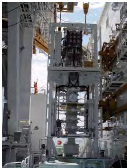
Figure 2. External view of *Chikyū*'s blow out preventer (BOP). BOP hangs from riser pipe attached to high-powered winches on ship's derrick and will be deployed onto seafloor through moonpool below drilling platform. Note person on left for scale.
