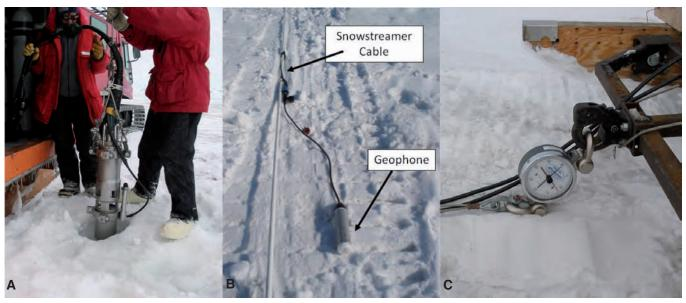
Figure 3. [A] Generator-Injector (GI) air gun being deployed through an auger hole in 6-m-thick sea ice; [B] Gimbaled geophone and the snow streamer cable; [C] Load cell attached to the back of the Thunder Sled and connected to a tow cable for the snow streamer (photos by R. Levy)
