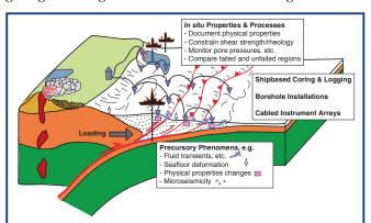
Figure 14. Schematic diagram of ocean drilling and borehole observatories to sample and measure in situ physical properties and mechanical state, and monitor transient phenomena that may be precursory to failure in actively deforming regions
