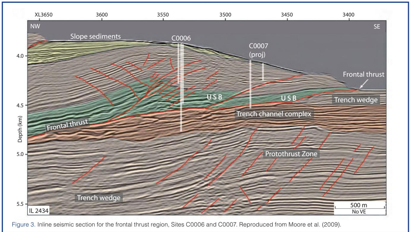
Figure 3. Inline seismic section for the frontal thrust region, Sites C0006 and C0007. Reproduced from Moore et al. (2009).
