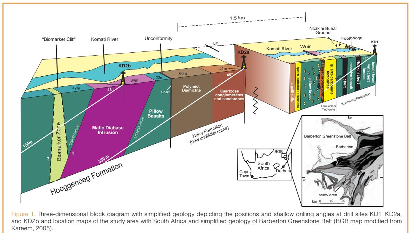
Figure 1. Three-dimensional block diagram with simplified geology depicting the positions and shallow drilling angles at drill sites KD1, KD2a, and KD2b and location maps of the study area with South Africa and simplified geology of Barberton Greenstone Belt (BGB map modified from Kareem, 2005).
