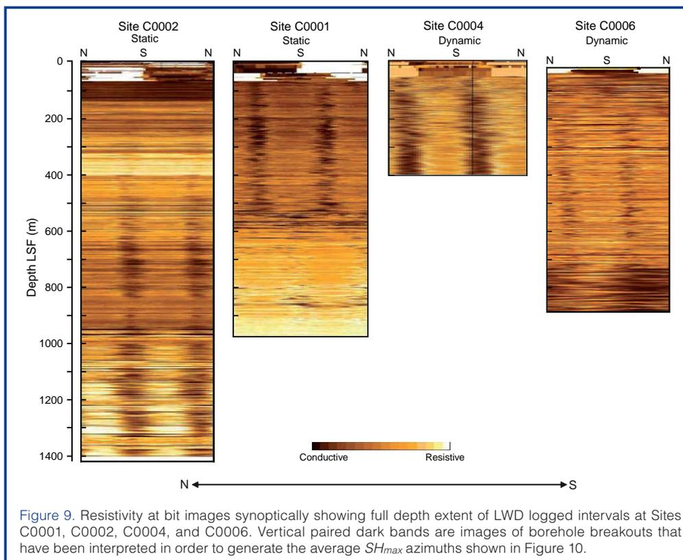
Figure 9. Resistivity at bit images synoptically showing full depth extent of LWD logged intervals at Sites C0001, C0002, C0004, and C0006. Vertical paired dark bands are images of borehole breakouts that have been interpreted in order to generate the average  $SH_{max}$  azimuths shown in Figure 10.
