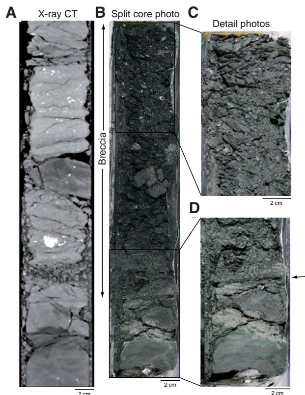
**Figure 5.** Fault core example from the frontal thrust region at Site C0007 (Expedition 316). Appearance of concentrated deformation in lower portion of frontal thrust fault Zone 3, at a depth of 438 mbsf. [A] CT image and [B] core photograph of finely brecciated hemipelagic mudstone (interval 316-C0007D-29R-2, 37–73 cm). [C] Close-up of finely brecciated interval. [D] Thin (2-mm-thick) dark layer (arrow) developed at base of finely brecciated interval.
