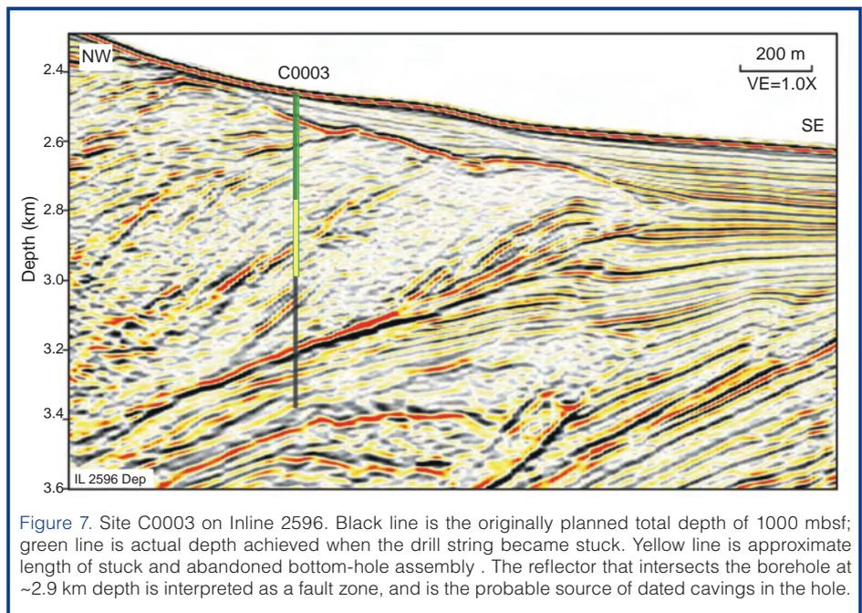
**Figure 7.** Site C0003 on Inline 2596. Black line is the originally planned total depth of 1000 mbsf; green line is actual depth achieved when the drill string became stuck. Yellow line is approximate length of stuck and abandoned bottom-hole assembly. The reflector that intersects the borehole at ~2.9 km depth is interpreted as a fault zone, and is the probable source of dated cavings in the hole.
