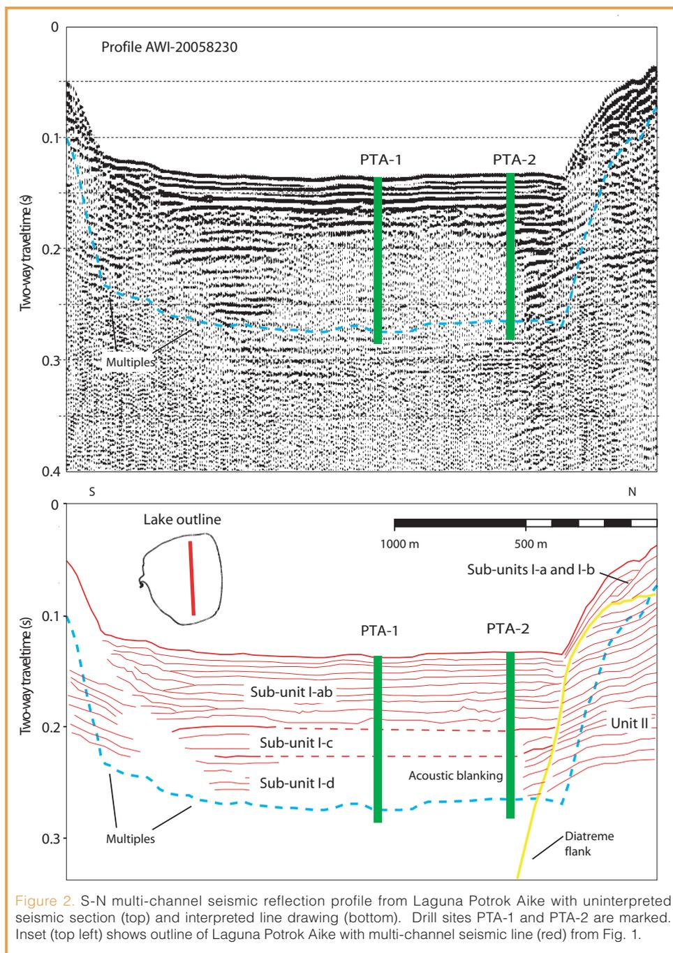
Figure 2. S-N multi-channel seismic reflection profile from Laguna Potrok Aike with uninterpreted seismic section (top) and interpreted line drawing (bottom). Drill sites PTA-1 and PTA-2 are marked. Inset (top left) shows outline of Laguna Potrok Aike with multi-channel seismic line (red) from Fig. 1.
