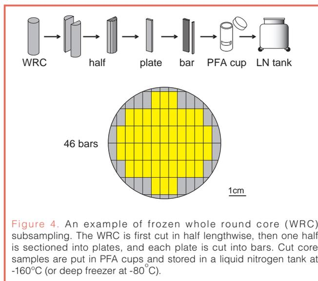
Figure 4. An example of frozen whole round core (WRC) subsampling. The WRC is first cut in half lengthwise, then one half is sectioned into plates, and each plate is cut into bars. Cut core samples are put in PFA cups and stored in a liquid nitrogen tank at  $-160^{\circ}\text{C}$  (or deep freezer at  $-80^{\circ}\text{C}$ ).
