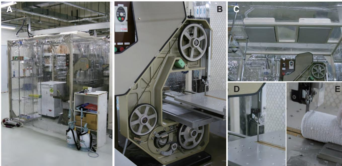
Figure 2. [A] Overview of the electric band saw system for microbiological frozen core. Motor-driven electric band saw machine [B] and  $-50^{\circ}\text{C}$  freezer is deployed in a clean booth equipped with two HEPA-filter units [C]. Diamond-tipped band saw cuts frozen core samples under clean conditions [D, E].
