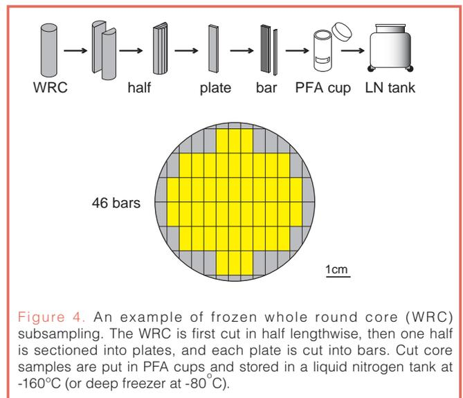
Figure 4. An example of frozen whole round core (WRC) subsampling. The WRC is first cut in half lengthwise, then one half is sectioned into plates, and each plate is cut into bars. Cut core samples are put in PFA cups and stored in a liquid nitrogen tank at  $-160^{\circ}\text{C}$  (or deep freezer at  $-80^{\circ}\text{C}$ ).
