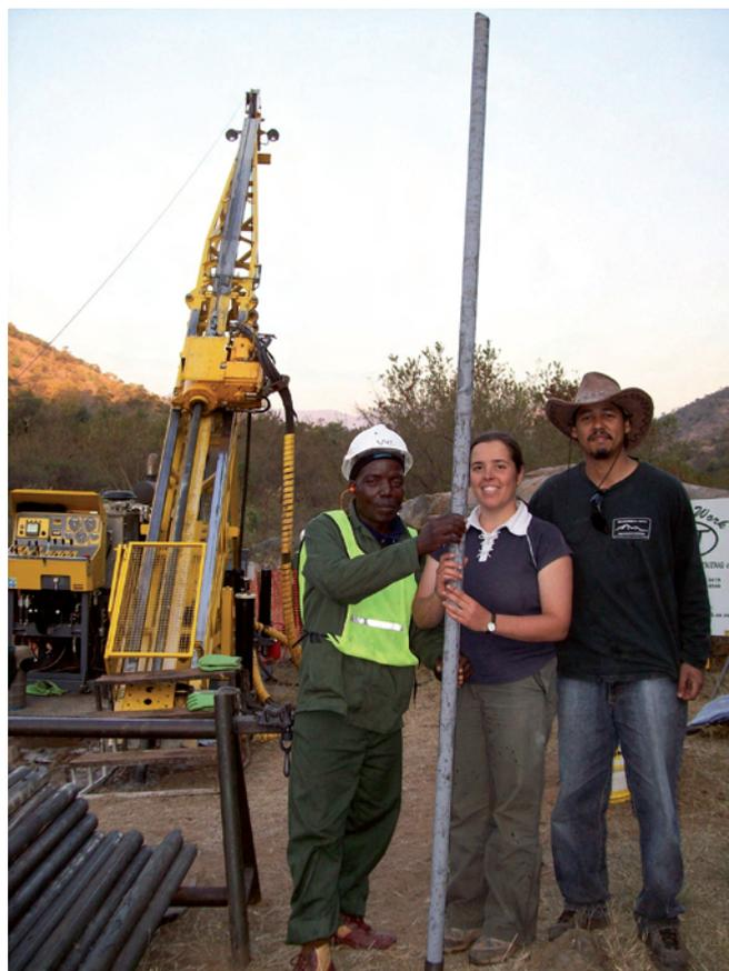
Figure 2. Drill rig aligned and set to drill at the shallowest possible angle (45°) relative to the dip and dip direction of the steep near-vertical orientation of the geological units along the Komati River. The >3-m-long rod is composed of basalt or diamictites.
