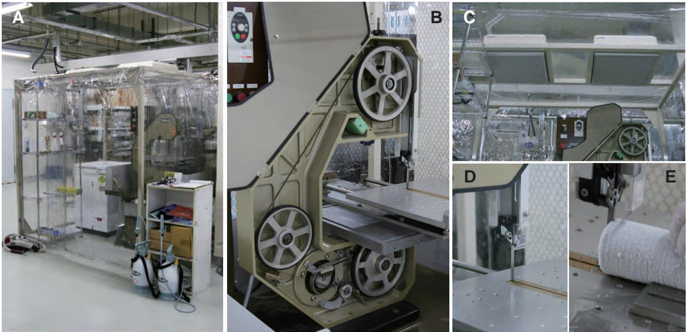
Figure 2. [A] Overview of the electric band saw system for microbiological frozen core. Motor-driven electric band saw machine [B] and  $-50^{\circ}\text{C}$  freezer is deployed in a clean booth equipped with two HEPA-filter units [C]. Diamond-tipped band saw cuts frozen core samples under clean conditions [D, E].
