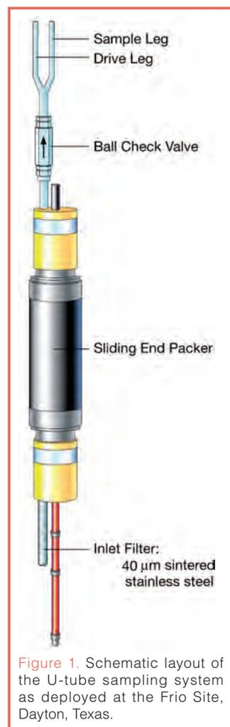
Figure 1. Schematic layout of the U-tube sampling system as deployed at the Frio Site, Dayton, Texas.
