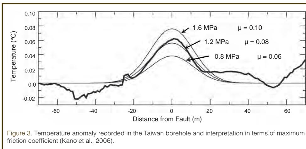
Figure 3. Temperature anomaly recorded in the Taiwan borehole and interpretation in terms of maximum friction coefficient (Kano et al., 2006).
