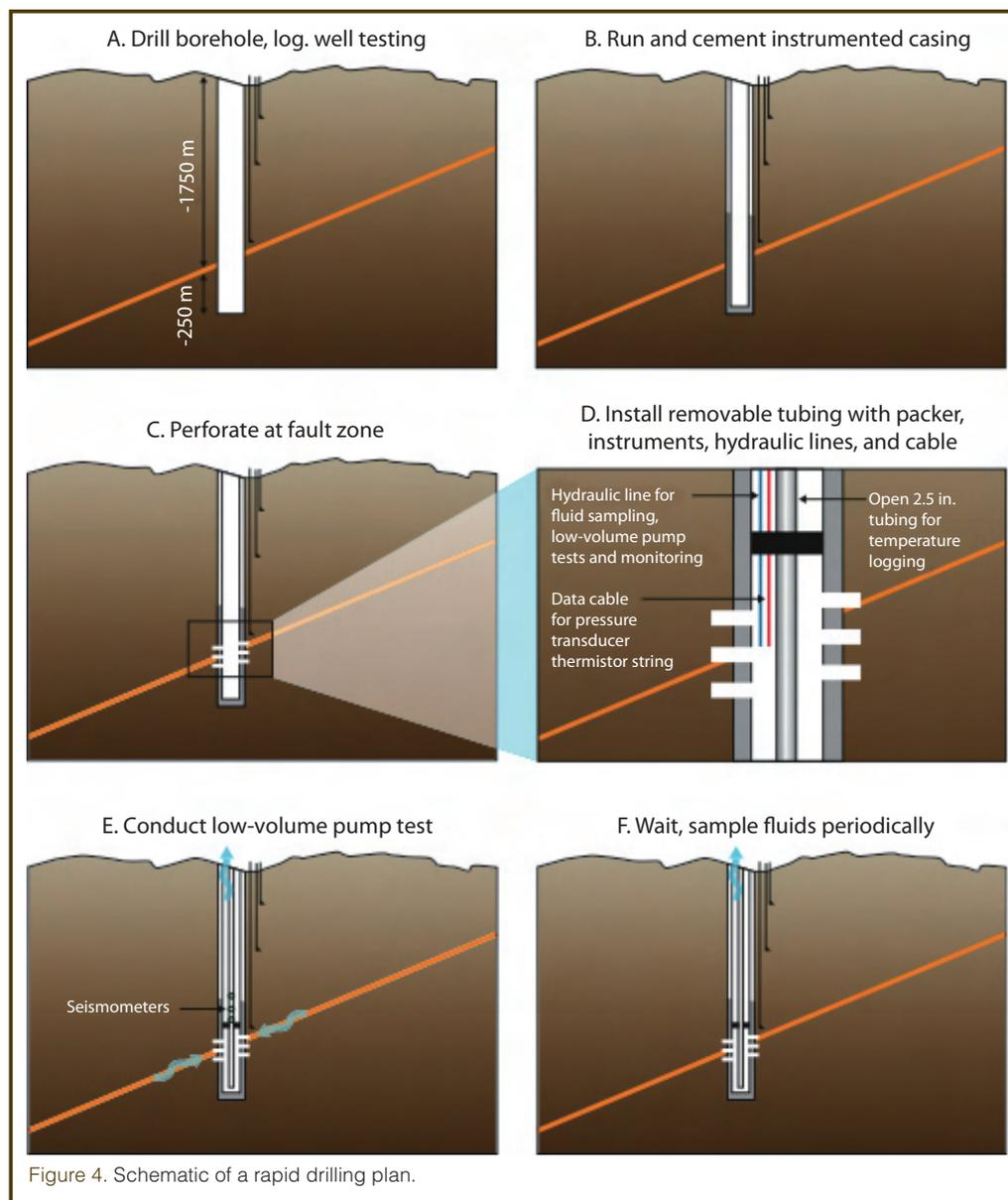
Figure 4. Schematic of a rapid drilling plan.
