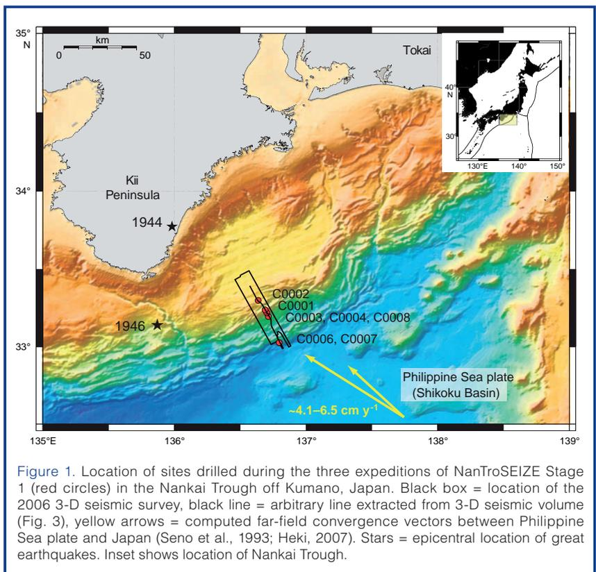
Figure 1. Location of sites drilled during the three expeditions of NanTroSEIZE Stage 1 (red circles) in the Nankai Trough off Kumano, Japan. Black box = location of the 2006 3-D seismic survey, black line = arbitrary line extracted from 3-D seismic volume (Fig. 3), yellow arrows = computed far-field convergence vectors between Philippine Sea plate and Japan (Seno et al., 1993; Heki, 2007). Stars = epicentral location of great earthquakes. Inset shows location of Nankai Trough.
