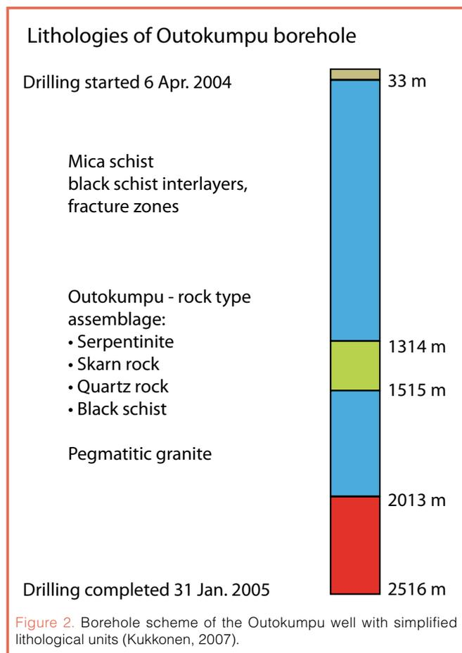
Figure 2. Borehole scheme of the Outokumpu well with simplified lithological units (Kukkonen, 2007).
