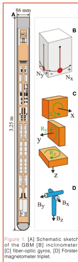
Figure 1. [A] Schematic sketch of the GBM [B] inclinometer, [C] fiber-optic gyros, [D] Förster magnetometer triplet.
