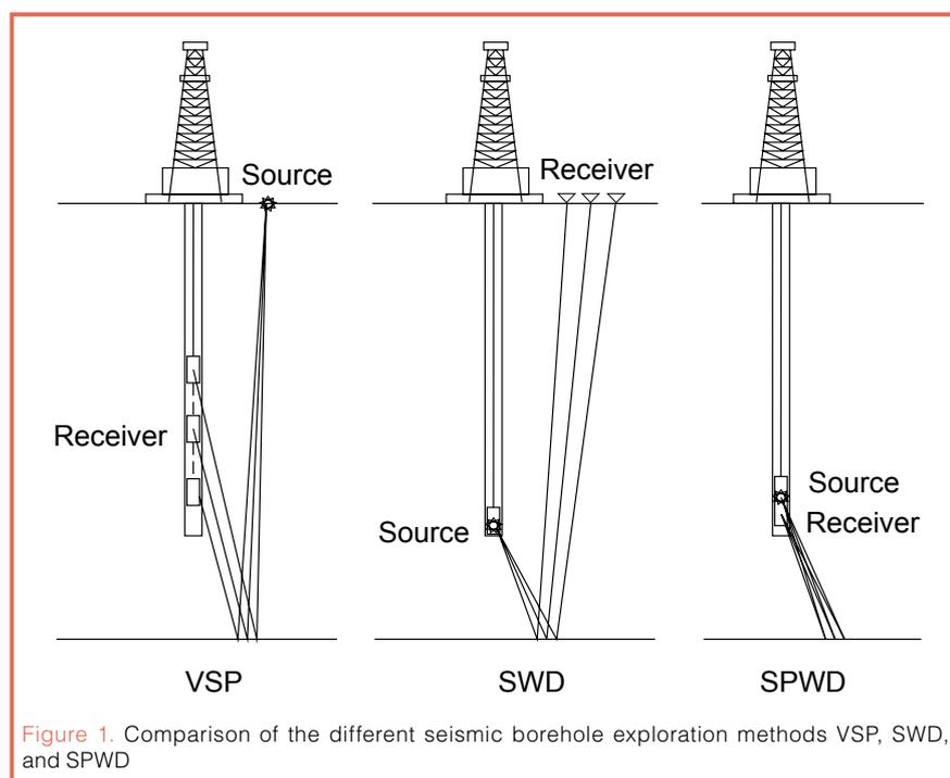
Figure 1. Comparison of the different seismic borehole exploration methods VSP, SWD, and SPWD
