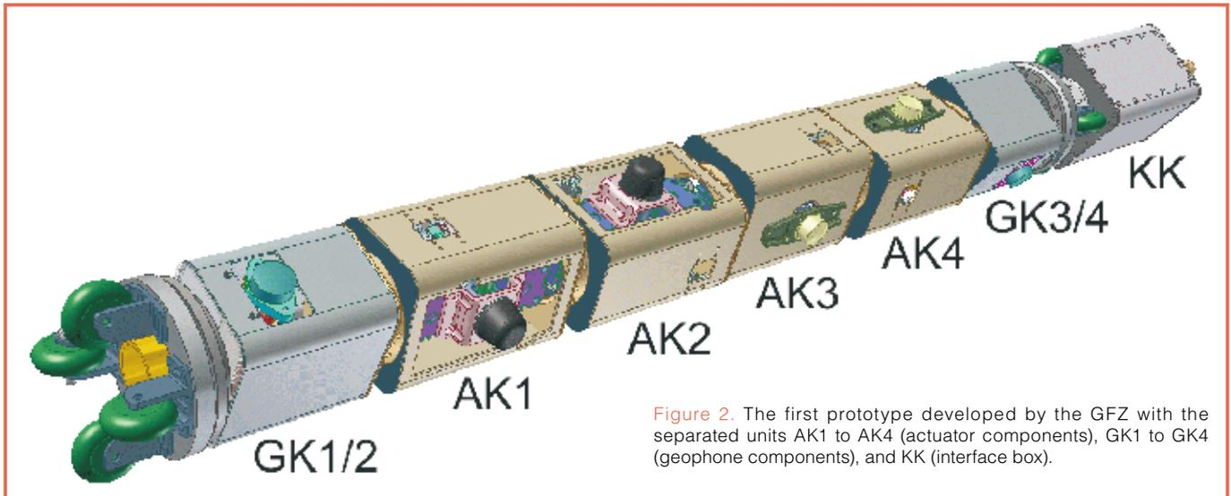
Figure 2. The first prototype developed by the GFZ with the separated units AK1 to AK4 (actuator components), GK1 to GK4 (geophone components), and KK (interface box).
