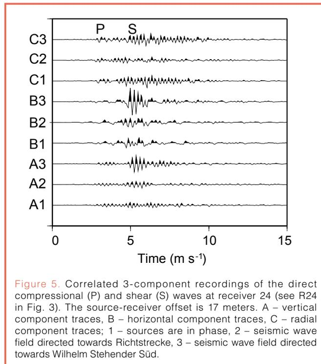
Figure 5. Correlated 3-component recordings of the direct compressional (P) and shear (S) waves at receiver 24 (see R24 in Fig. 3). The source-receiver offset is 17 meters. A – vertical component traces, B – horizontal component traces, C – radial component traces; 1 – sources are in phase, 2 – seismic wave field directed towards Richtstrecke, 3 – seismic wave field directed towards Wilhelm Stehender Süd.
