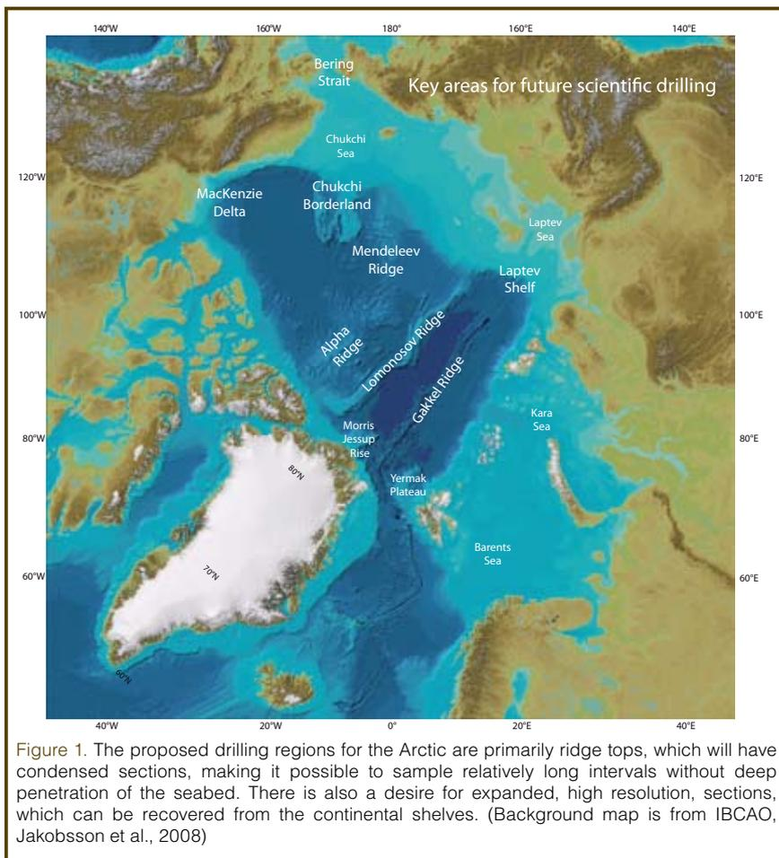
Figure 1. The proposed drilling regions for the Arctic are primarily ridge tops, which will have condensed sections, making it possible to sample relatively long intervals without deep penetration of the seabed. There is also a desire for expanded, high resolution, sections, which can be recovered from the continental shelves. (Background map is from IBCAO, Jakobsson et al., 2008)
