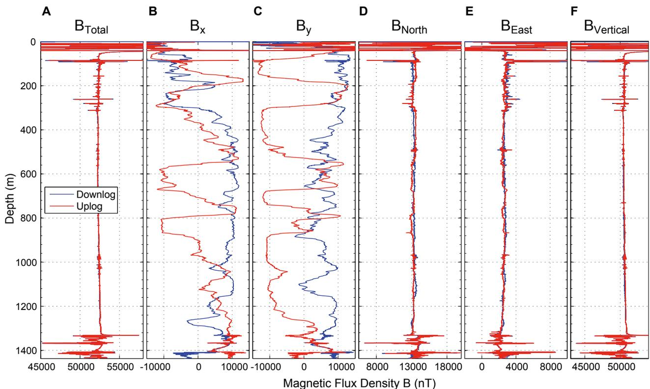
Figure 3. [A] Total magnetic flux density, [B and C] horizontal components before reorientation (internal tool coordinates  $xyz$ ), [D–F] magnetic flux density after reorientation with geographic coordinates North, East, Vertical.
