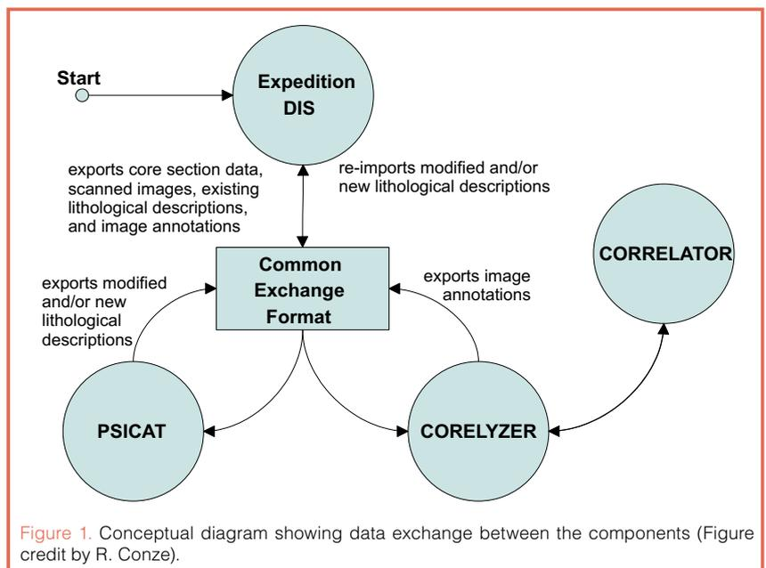
Figure 1. Conceptual diagram showing data exchange between the components (Figure credit by R. Conze).
