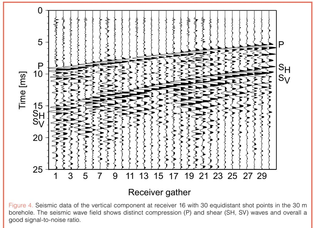
Figure 4. Seismic data of the vertical component at receiver 16 with 30 equidistant shot points in the 30 m borehole. The seismic wave field shows distinct compression (P) and shear (SH, SV) waves and overall a good signal-to-noise ratio.
